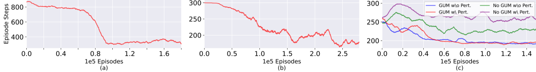
Figure 2: Task completion times during training for learned policies averaged over 10 trials (a) bi-pushing, (b) bi-reorienting, and (c) bi-gathering tasks. Note that less task completion time means better performance. Our proposed goal-update mechanism (GUM) in the bi-gathering task resulted in improved performance: the blue and red plots (with GUM) show reduced numbers of time steps required to achieve the task in one episode, under both perturbed and unperturbed conditions, compared to the green and purple plots (without GUM).
